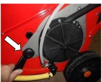
2) Loosen the black turbine lock knob as shown at the bottom of the image to the left by turning counter-clockwise. Now the turbine drive assembly and bracket will slide down and away from the sprinkler cart (as shown by white arrow) to disengage the turbine drive gears. Re-tighten the knob to hold the turbine drive gear away from the drum gear. Drum will now spin freely allowing sprinkler cart to be pulled out.
