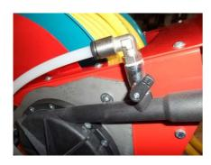
9) Adjust the speed of cart retraction by moving the bypass lever or speed control lever in the directions shown by the arrow. Closing this valve will increase the retraction speed and opening the bypass valve will slow down the retraction speed.
