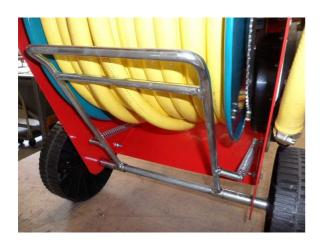
The hose tensioner is fitted when the wheels are assembled to the chassis.
