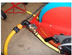
7) Attach supply hose provided to the inlet of the machine and lock into place as shown
