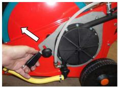
5) Re-engage the turbine assembly by loosening the black knob again and sliding the turbine bracket back into place as shown by white arrow, so that the drive gears mesh. Tighten the black lock knob again to hold the turbine in place.
