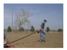
3) Sprinkler cart may now be pulled out by hand. **IMPORTANT:** Pull the sprinkler cart out in a straight line from the machine to allow the tube to wrap back onto the drum straight. Never make sharp turns with the polyethylene hose and always leave one or two wraps on the drum to keep from pulling the tube off of the drum.
