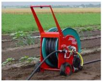
1) Push the machine to the desired location. Position the machine with the sprinkler cart facing the direction to be irrigated. Insure that the machine is sitting level in order for the tube to wrap properly.
