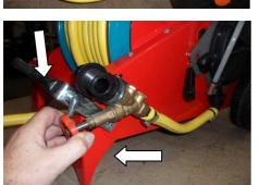
IMPORTANT: Before proceeding, try turning the drum by hand to make sure it is locked in gear. It should be locked and will not turn.
