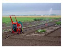
8) Turn on the water source to the MMR20. The sprinkler equipped with the MMR20 can be set to water a full circle pattern or any part of a circle. It is generally recommended to water a three-quarter circle pattern behind the cart, away from the direction of travel. The MMR20 is equipped with a pressure regulator at the inlet to maintain system pressure at no more than 60 psi.
