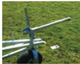
End of run out of gear mechanism and steering assembly.
