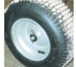
Flotation tyres for low ground pressure.
